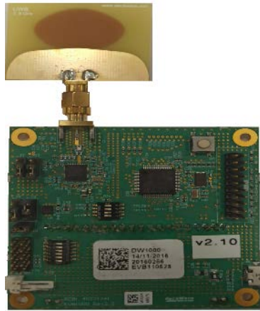
Figure 4-2: EVB1000 Module Used as a UWB Node.
